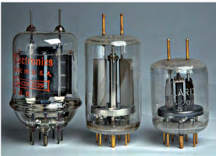
Fig. 4: Comparing the American 3E29 double-valve on the left, alongside the European style QQV03-20 and QQV06-40A 'siamese-twinned' valves.
