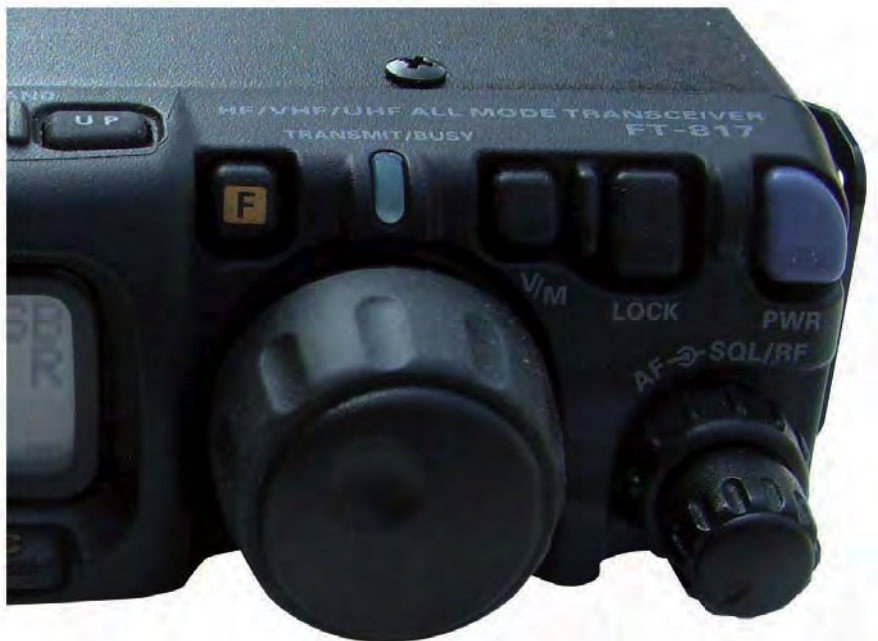
Fig. 3: The right-hand side of the front panel showing the yellow F button above and to the left of the main tuning control.
