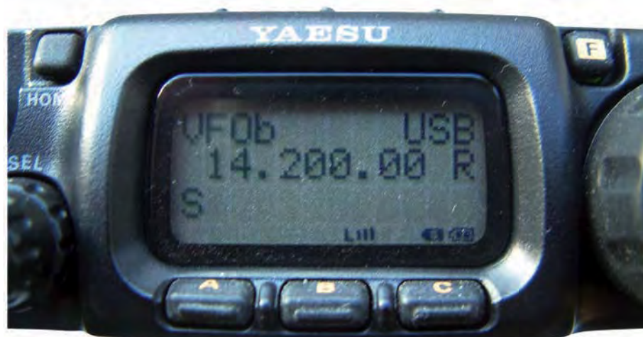
Fig. 4: The display showing the dual v.f.o. options.
