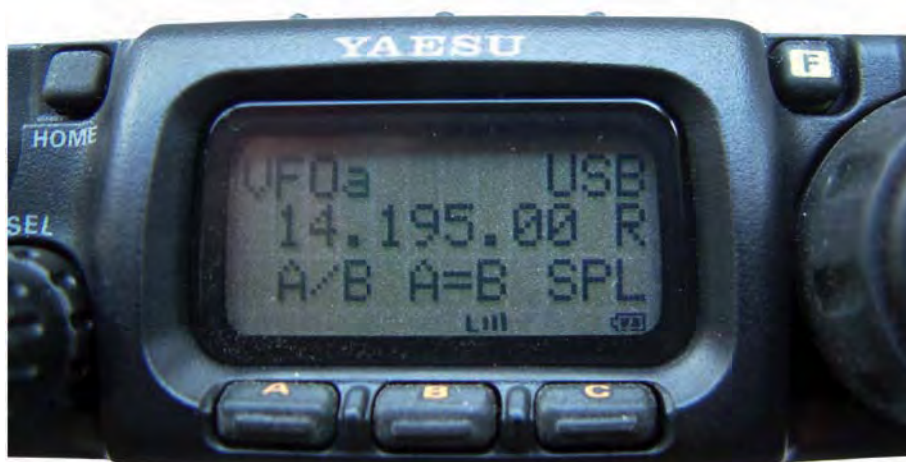
Fig. 4: The display showing the dual v.f.o. options.
