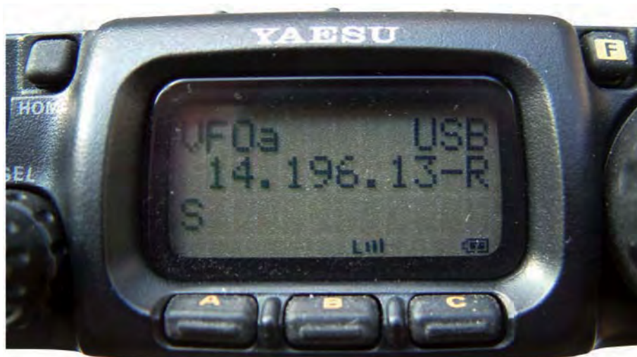
Fig. 2: The display showing the “-” sign between the 3 and the R indicates that the clarifier is in use. The large R indicates that the rear antenna socket is enabled.
