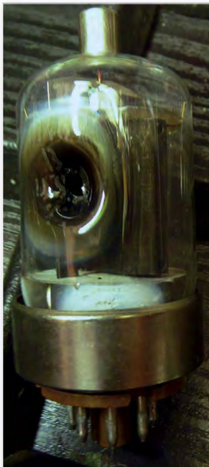
Fig. 2: Lack of ventilation can cause overheating of valve envelopes leading to an 'implosion' as shown on this example – it ruins the valve, of course!
