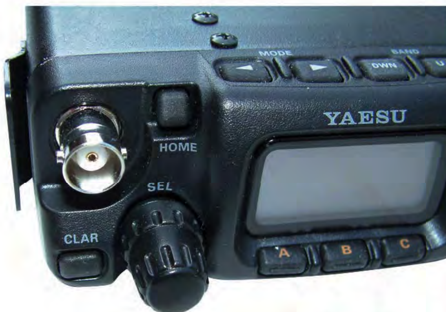
Fig. 1: The left-hand side of the front panel showing the clarifier button (CLAR) and SEL rotary control.
